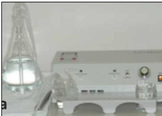
**Figure 1a:** MOZO Generation. Medical ozone generator with water flask for producing ozonated water.
