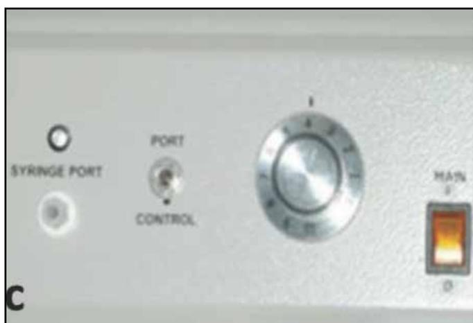
**Figure 1c:** Control panel with syringe port and corona discharge regulator. The concentration of ozone in oxygen is controlled by adjusting the rate at which oxygen flows past a corona plasma discharge with a specific voltage being generated.
