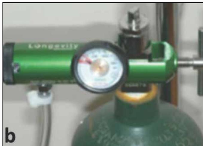
**Figure 1b:** Oxygen tank with pediatric regulator that can deliver oxygen flow rates down to 1/32 of a liter per minute.
